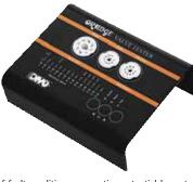
pre-amp valves for a wide range of fault conditions, preventing potential harm to other components of your amps. The unit has (1) octal and (2) 9- pin valve sockets. In approximately 2 minutes, it performs an extensive series of tests on valves' heater filaments (short circuit, open circuit and tolerance check), heater cathode insulation (leakage and short circuit), heater current abnormalities, amplification factor, voltage gain, power gain, and many more.
