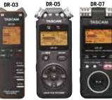
(except for DR-07), and the ability to record in WAV or MP3 formats. The DR-03 features stereo omni condensers and a built-in desktop stand. The DR-05 also features stereo omni condensers as well as a chromatic tuner and editing functions. The DR-07 has stereo
