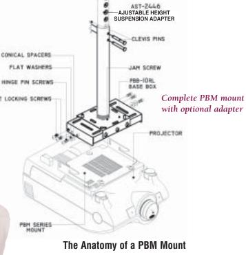
Our PBM mounts fit projectors of various sizes and weights. Each mount is designed with a different base box to accommodate these variables.
