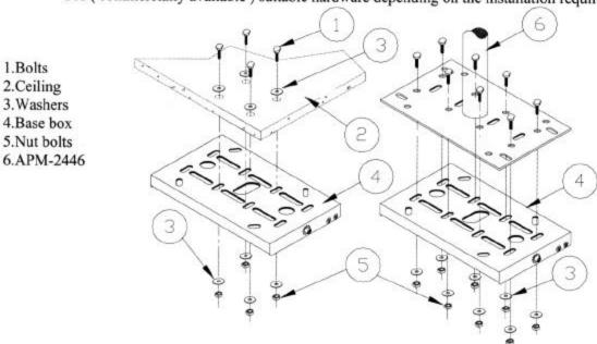
**NOTE:** If **ASA-2446** adjustable height suspension adapter is a part of the installation, securely install the adapter to the ceiling at this time. (Refer to its installation instructions.)
