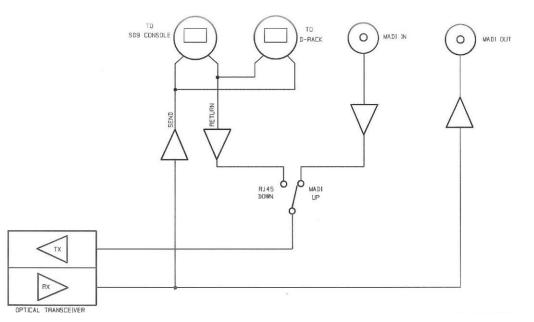
The unit is equipped the RJ45 mixer and rack connections (i.e. in/out or out/in) to suit the D-Rack family of interfaces and the SD9 / SD11 series of mixers
