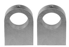
The Mega-Truss Tee Clamp is great for holding a pipe to the end of a truss for holding light fixtures. Sold in pairs and provided with  $5/8'' \times 1-1/4''$  Hex head bolts to fasten through the standard truss bolt holes. I/2-13 socket set screw for locking pipe into position. CNC machined from solid 6061T-6 aluminum with 5/8''-11 tpi internal threads for mounting.
