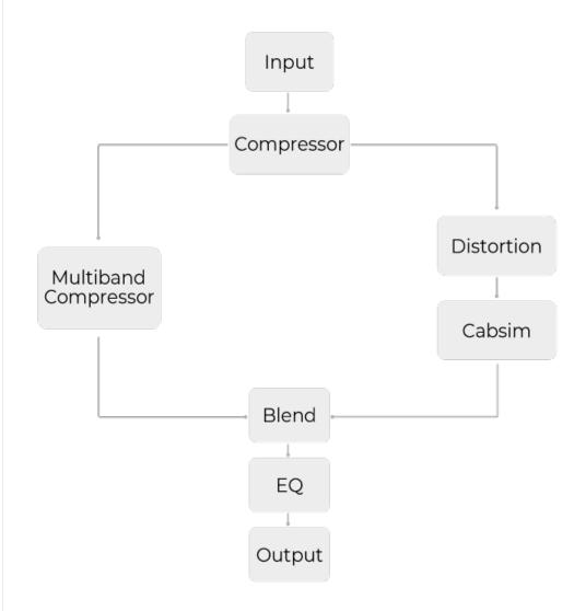
**Compressor**: This control allows setting the input gain of the compressor that will translate into how much the signal is compressed while our intelligent make-up gain algorithm keeps the output of the compressor at usable levels. The compressor has 5 ratios available: 4:1, 8:1, 12:1, 20:1 and ALL IN.
