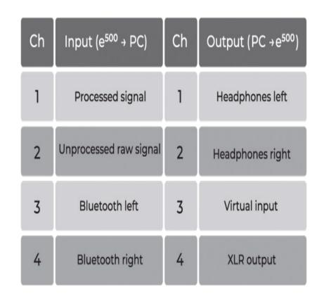
The processed signal input is the signal at the very end of the signal chain.
