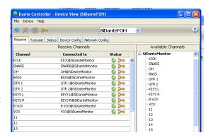
Available Channels: On the right pane of the window, lists the Tx channels from other devices that are available for subscription by the current device. You may drag and drop Available Channels to Receive Channels.
