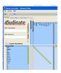
**Device Status** – Displays information about discovered Dante devices; double click a device name to enable its configuration.
