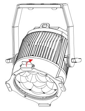
Align the gel frame holder on the frame, then re-install the four (4) screws to secure in place. Flip the latch open.
