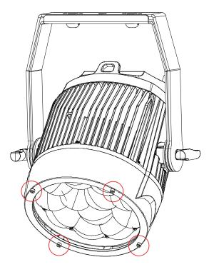
1. Remove the four (4) screws around the frame of the fixture's lens.
