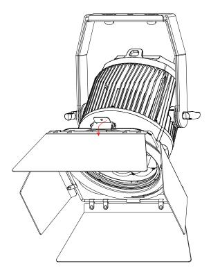
6. Flip the latch closed to secure the gel frame and barndoors in place.
