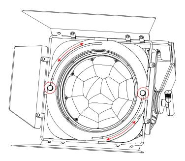
5. Align the semi-circular slots on the front of the barndoors with the two screw holes located on the tabs of the gel frame holder, and loosely re-install the included thumb screws. Twist the barndoors to adjust their position, then tighten the thumb screws to secure in place.
