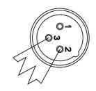
A DMX512 terminator reduces signal errors, avoiding most signal reflection interference. Connect PIN 2 (DMX-) and PIN 3 (DMX+) of the last fixture in series with a 120 Ohm, 1/4 W Resistor to terminate the DMX512.
