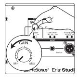
3. Turn the output of your audio source (audio interface, mixer, or speaker-management device) to its lowest setting.
