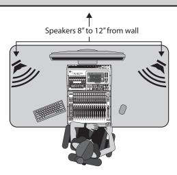
Before placing your studio monitors in your mixing environment, position your desk or monitor stands so that your speakers will be at least 8 to 12 inches away from walls and corners. This will be adequate to prevent sound waves from hitting the wall and reflecting back to you, causing phase cancellation and other potentially harmful acoustic interactions. This might not always be possible, and there are some ways to mitigate cramped mixing spaces.
