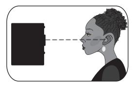
Ideally, near-field studio monitors like the Eris Pro-Series should be placed so that the high-frequency drivers (commonly known as 'tweeters') are at the same height as your ears when you are seated in the mix position.
