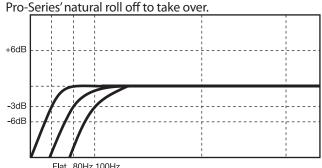
**Power User Tip:** If you are using a subwoofer that doesn't feature a variable low pass filter, like the PreSonus Eris Pro Sub 10 provides, you will use this control to set the crossover point for your 2.1 system. **For information on configuring a 2.1 system in the studio, please visit** My.PreSonus.com.
