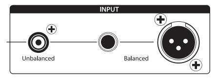
**Line-level Inputs.** The Eris Pro-Series monitors provide a choice of three line-level input types: balanced XLR, balanced ¼"TRS, and unbalanced RCA. Do not connect more than one source to your Pro-Series monitors simultaneously.
