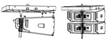
As shown in the picture, in flown installation, the use of the pins and of the rear bracket of DRK-210 make the assembly with the first element of the line-array simple and safe.
