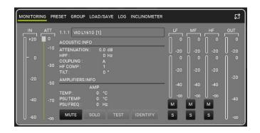
The software which must be used in case of remote control is dBTechnologies AURORA NET. This software can control different speakers in different configurations.
