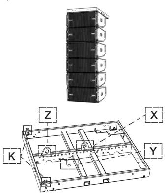
The DRK-210 fly-bar allows different configurations, flown or stacked, for the professional stage use. It has 2 load adaptors (X, Z) for the use of up to two different rigging motors, one rear bracket (Y) specifically designed for the flown installation, and 2 movable bars [K] for stack mounting. The maximum admitted number of cabinets in different configurations depends on various parameters, like VIO L1610 splay angles and DRK-210 tilt.
