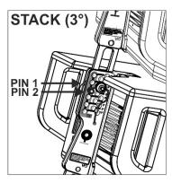
allowed by the first pin, and fasten the second pin in the related "ANGLE LOCK" position. Then release the upper enclosure and check that the movable arm leans on the second pin, fastened in the correct position.
