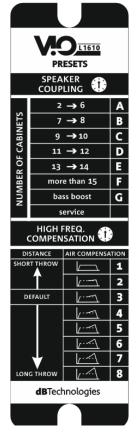
mainly on low frequencies, and it can be set in 6 positions, depending on the number of elements of line-array.
