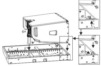
In stacked installation (for example a line-array stacked on a S318 sub), the use of the pins, of the rear bracket of VIO-L1610, and of the 2 movable bars of DRK-210, as shown, make the assembling quick and easy.
