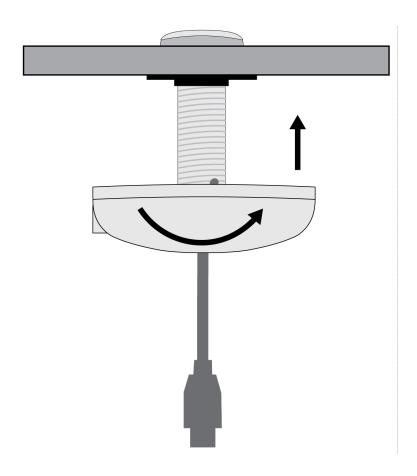
5. Connect the 8-pin power cable to the power connector on the base.
