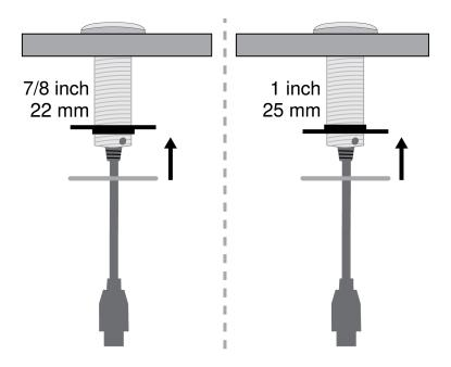
4. Slide the base onto the tube and tighten it by hand until it is snug against the table. You may want to hold the top of the mute button as you tighten the base to keep the mute icon correctly positioned on the table.
