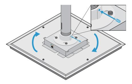
7. Connect the Ethernet cable to the microphone.
