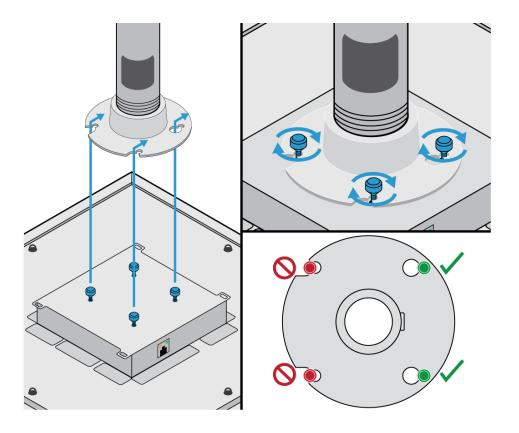
6. Rotate the microphone to your preferred position. Tighten the VESA bracket's set screw with the Allen key to lock the position.
