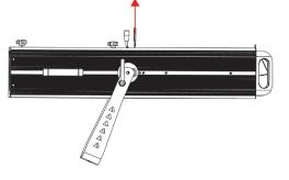
2. Unscrew the retainer screw from the Gobo Holder.
