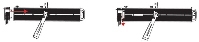
2. Tighten the thumb screws to secure the 4-slot Boomerang in place.
