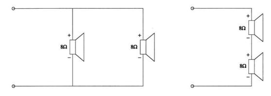
**Figure 4b**: Simple parallel connection:  $4\Omega$ .
