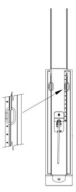
The i9 MAB is attached to the cabinet as shown with the supplied hex socket screws and washers supplied. Remove the original M10 counter sunk screws from the top and bottom of the i9, position the bracket with the marked hanging holes to the top of the cabinet, then replace these counter sunk screws with the hardware supplied.
