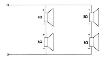
Figure 4d: Series Parallel Combination:  $8\Omega$
