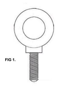
The Tannoy VS18DR loudspeaker can be flown with high quality VEB M10 eyebolts with collar to BS4278:1984. The loudspeaker is equipped with internal steel braces, which also double as the flying points, and accept VEB M10 eyebolts.
