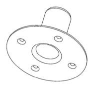
The Tannoy VS18DR loudspeaker is fitted as standard with a blanking plate on top of the cabinet. However, should you ever wish to mount a V series cabinet above the VS18DR using standard 35mm tube, this blanking plate can be quickly and easily removed and replaced by a VTH pole mount. The same screws that secure the blanking plate should be used to secure the VTH in position.
