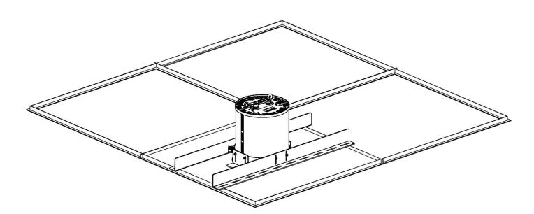
4. Install the entire assembly back into the ceiling at the desired location, making sure that the ends of the grid support brackets are resting firmly on the support grid for the ceiling. Secure the grid support brackets in place using the appropriate hardware.
