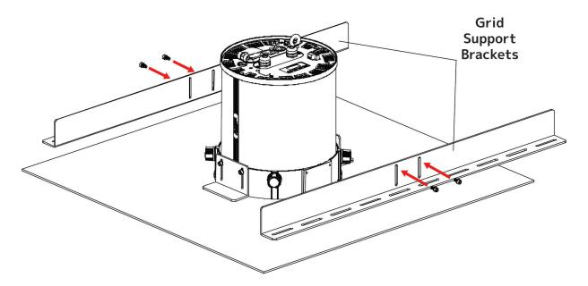
3. Attach the grid support brackets to the trim ring using the included screws.
