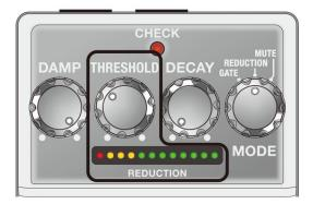
6. Use the [DAMP] knob to adjust the amount of the gate and reduction effect.
