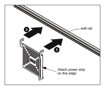
**CAUTION:** Do not bump CSA100 or its attached components. If bumped from below the CSA100 may dislodge from the rail.
