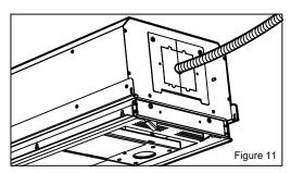
(5) Attach complete outlet box configuration to projector mount plate as shown below in figure 12. Secure by re-attaching nuts removed in Step 1.
