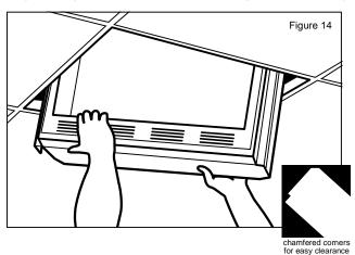
(2) Rotate and drop box to gently rest into place onto drop ceiling framework.
