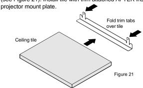
Finish frame assembly by opening four latches in door panel dropping panel down. Slide tile (cut to size) into location.
