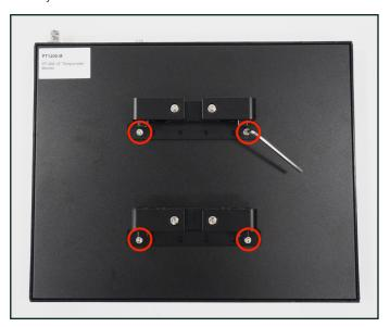
**Step 2**Using the larger hex key loosen the rod clamps.
