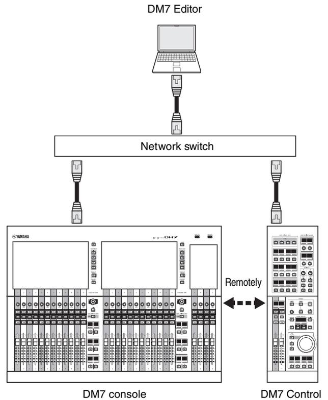
You can use this product (which is connected via a network cable) in another location on the network, remote from the DM7 console.
