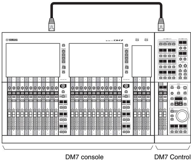
You can link up and affix this product to the DM7 console using joint metal brackets. (“Linking with the DM7 Console” → page 12)
