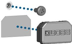
3. Attach the BT-DUAL and fasten the screw that you removed in step 2 in place.
