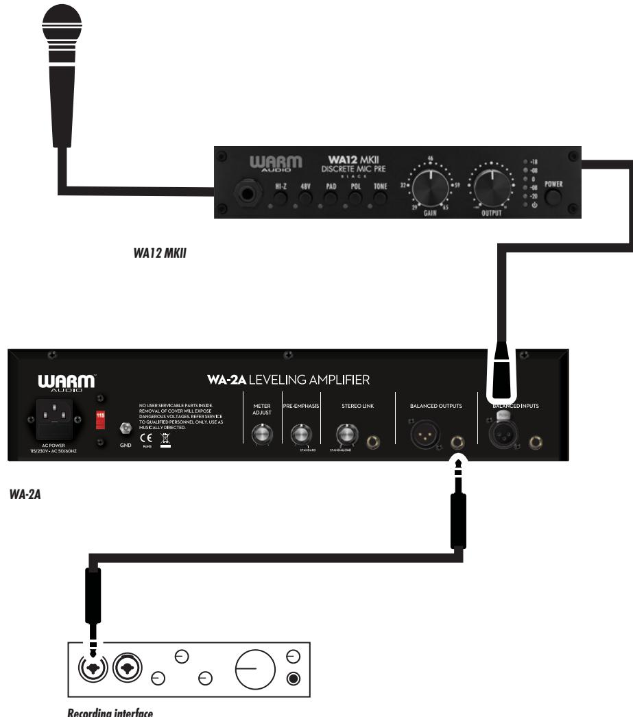
In this diagram the WA12 MKII is used as a mic preamp to capture a microphone signal which then feeds into the WA-2A Compressor. After leaving the WA-2A, the signal enters the recording interface.
