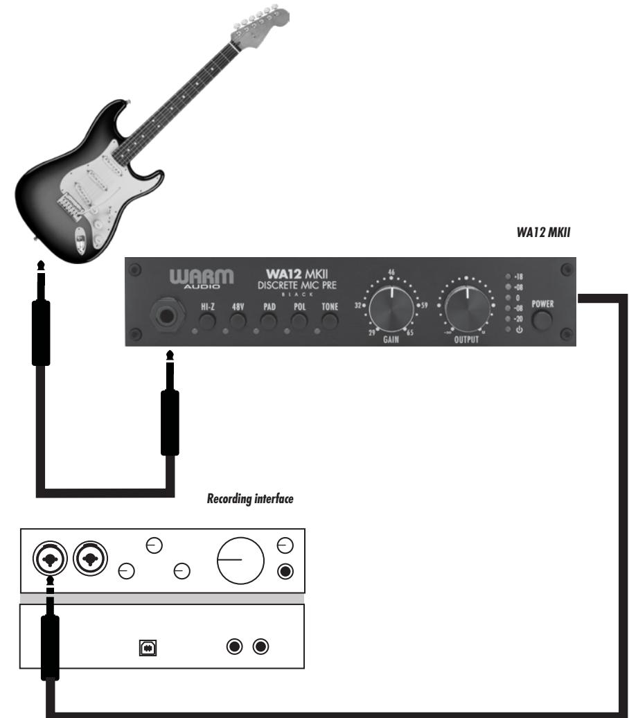
In this diagram, the WA12 MKII is used as an active instrument DI to capture an electric guitar and bring the signal into a recording interface.
