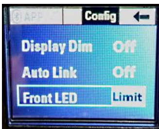
Fig. 55 Front LED parameter set to Limit
