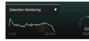
Click on the arrow in the lower left corner to expand the Distortion Monitoring display. The spectral representation indicates the amount of distortion in bright red for different frequency regions.
