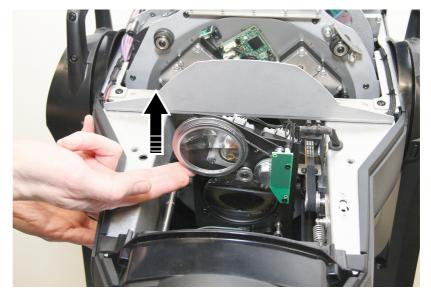
Figure 21: Lifting up the prism
