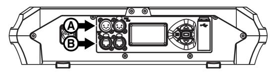
Figure 8: Data connections
