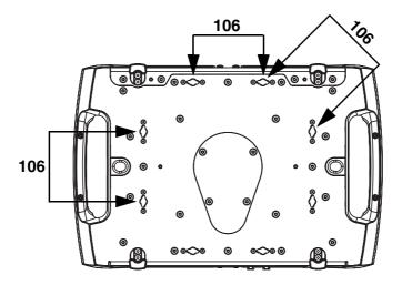
Figure 3: Omega bracket mounting points
