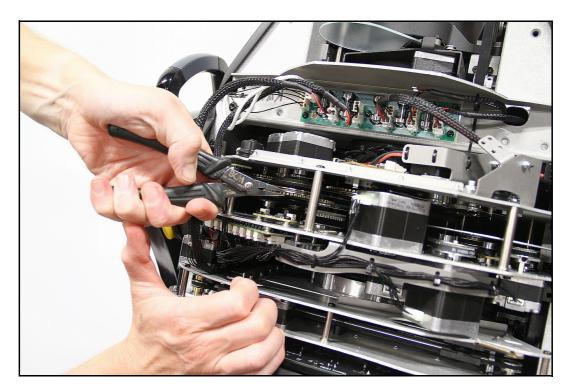
Figure 15: Removing a goboholder from Gobo Wheel 1
