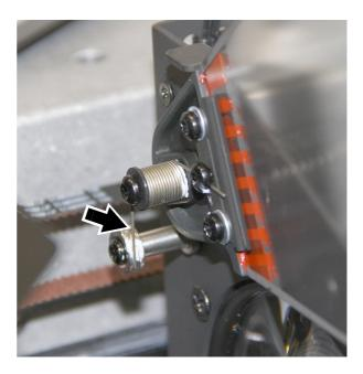
Figure 28: Frost filter spring
