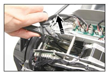
Figure 16: Removing a gobo from Gobo Wheel 2
