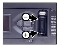
Figure 10: Battery replacement
