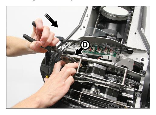
Figure 17: Reinstalling a goboholder
