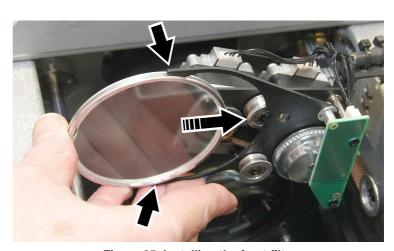
Figure 25: Installing the frost filter
