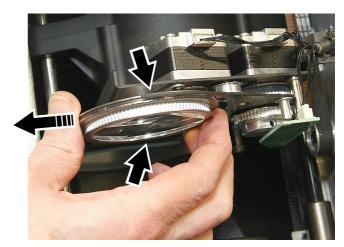
Figure 24: Removing the prism
