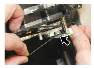
Figure 23: Disengaging the prism drive belt
