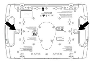
Figure 6: Safety cable attachment points
