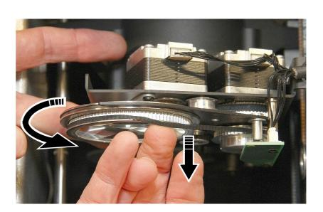
Figure 22: Disengaging the prism drive belt
