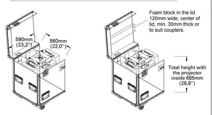
The SiP insert must be inserted into a flight case for 2x MAC Encore: P/N 9155048
