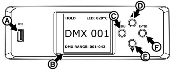
A - USB port B - LCD display C - Menu button D - Up button E- Down button F - Enter button
