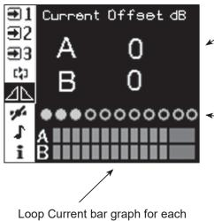
Loop Current bar graph for each channel. Shows Loop output current in 2dB steps from >-20dB to 0dB in green. Red = clipping Current Offset value adjusted by rotary control. Counter clock-wise reduces channel A. Clock-wise reduces channel B. Adjustment is from 0 to -10dB on either channel. Further adjustment turns that channel off and disables loop test for that channel.
