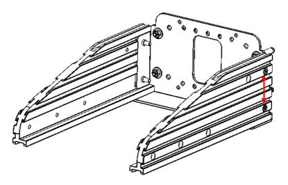
4. Place the round rod in between the left and right brackets then secure it in position by fastening two *M5x20 nickel plated hex* socket cap screws to the respective holes on the brackets as shown in the diagram below.
