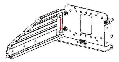
3. Assemble the right bracket to the wall plate with two *M5x20 nickel* plated hex socket cap screws as shown in the diagram below.
