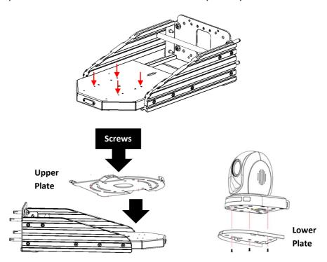
Mount the PTC-150 to the WM-11 as shown in the diagram below.
