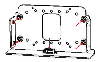
Please note that you can use the bubble level meter to make sure that the wall plate is properly aligned. If the bubble is at the center, the wall plate is horizontally aligned (perfectly levelled). If the bubble is on either side, the wall plate is tilted to the sides. 2. Assemble the left bracket to the wall plate with two *M5x20 nickel plated hex socket cap screws* as shown in the diagram below.
