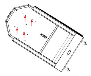
Secure your PTR-10/10T with four *M3 x 10mm screws and spring* washers.
