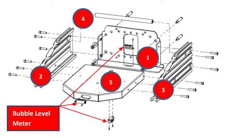
First mount a bubble level meter to the wall plate using two M2.5 screws. Align the wall plate with the four holes drilled in Pre-Work then use four expansion bolts to secure the wall plate. See the diagram below.
