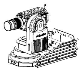
If after installation, the PTR-10/10T vibrates, you may enhance the installation by securing the base with four M3 x 8mm screws. The additional screw holes are depicted in the diagram below.
