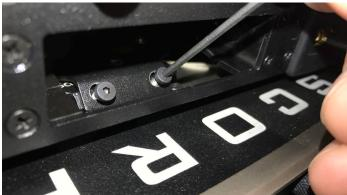
**STEP 2** Gently raise the SL-2 and slide towards the rear of the unit. Lift up and over the silver mounting screw circled in red.
