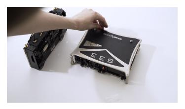
**STEP 4** Align the SL-2's bottom panel hooks with the Rear Keyhole Pegs on the 833/888. The SL-2 should be tilted with the front panel slightly higher than the rear. Take care not to bump the SL-2 expansion connector against the 833/888 top panel. Once the SL-2's Bottom Panel hooks and Rear Keyhole Peg's machined grooves are aligned, slide the SL-2 towards the front panel.
