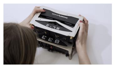
**STEP 6** Using the supplied 2 mm Allen Wrench, secure the SL-2 to the 833/888 top panel with the two captive screws as shown in the image below.
