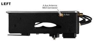
A & B AUX ANTENNA MCX CONNECTORS Distributes Antenna A and B to external receivers.
