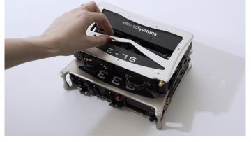
**STEP 3** Gently raise the SL-2 and slide slightly forward to disconnect from the mixer-recorder.
