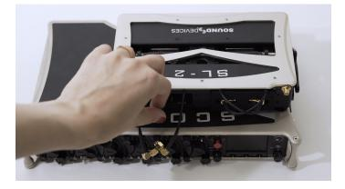
**STEP 8** Secure the SL-2 to the Scorpio Front Bracket with two 6 mm screws using the supplied 2 mm Allen Wrench.
