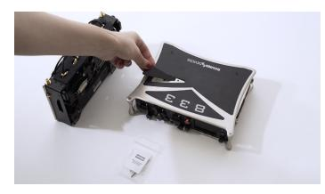
**STEP 2** Using a #4 Phillips Screwdriver, remove the two black phillips screws from the Scorpio top panel as shown in the image below. Keep these screws in a safe place as they need to be re-installed if the SL-2 is removed from the 833/888.
