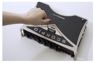
**STEP 4** Remove the safety mount from the top panel of Scorpio.
