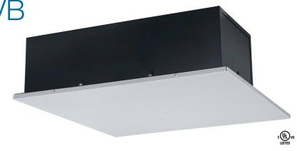
LT SERIES SPEAKERS are pro systems made for quick installation in suspended lay-in tile ceilings. The 2x2 assembly replaces a 2x2 ceiling tile. This model features a premium 8-inch coaxial driver, 70V 8W transformer, 2x2 grille with subplate and 0.8 cu.ft. volume backbox.
