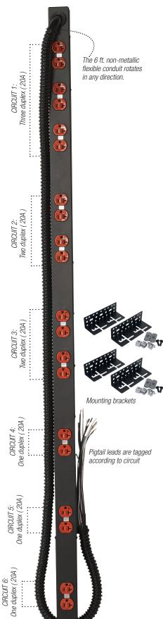
Six-circuit power strip with insulated ground (isolated ground or I.G.) receptacles is made to safely power equipment in installations that require multiple AC power circuits. Features 20 receptacles (10 duplex). Requires 35U panel space (minimum).
