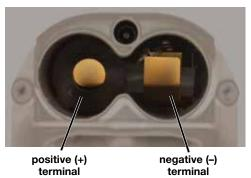
Note: It is possible to install the batteries backward and close the battery door, but the batteries will not make contact and the unit will not power up.
