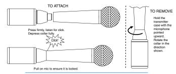
NOTE: Do not hold or apply any pressure to the microphone body while trying to remove it, as this may prevent the latch from releasing.
