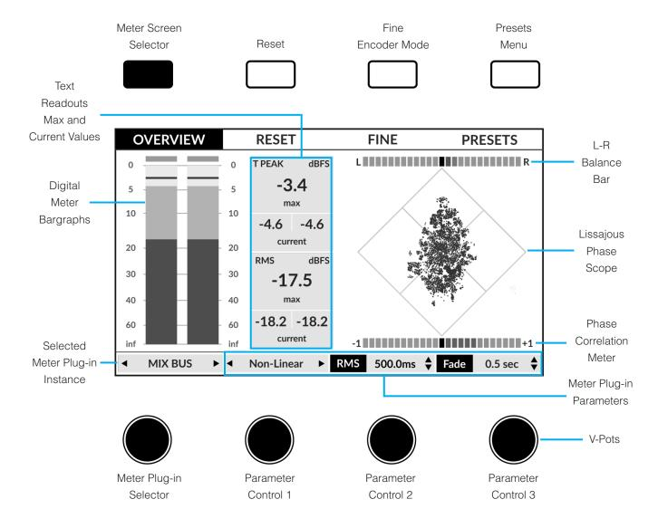
Meter Screen Selector - Press the key to toggle through the 3 different meter screens: Overview, Analogue and RTA.
