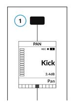
The Pan Key is located on the Soft Key abvove the Small LCD Screen
