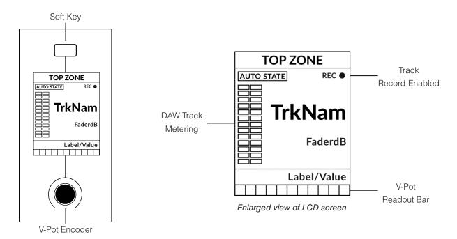
**Top Zone** - Provides a label for the function assigned to the soft key directly above.
