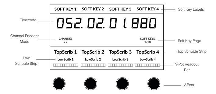
Soft Key Labels - Labels for the functions assigned to the soft keys directly above.
