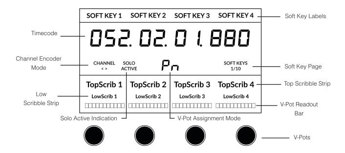
Soft Key Labels - Labels for the functions assigned to the soft keys directly above.
