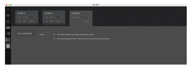
**UF1 follows selected Plug-in Mixer Channel Strip instance** - With this setting enabled, UF1 will always follow the selected 360°-enabled channel strip instance, which effectively means UF1 and UC1's selected channels are linked together. Disabling this setting, is the same as engaging the **MASTER** key on UF1 which means that UF1 can control a different 360°-enabled channel strip to the one that UC1 is controlling.
