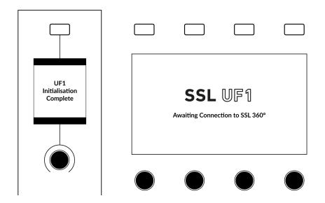
'UF1 Initialisation Complete' means that the UF1 hardware boot sequence has completed. 'Awaiting Connection to SSL 360° means that UF1 is waiting for the SSL 360° software to start running on the computer. You may see this message appear when logging onto your computer, before the operating system has finished loading your user-profile and start-up items. You may also see this message if you are yet to plug a USB cable from your UF1 into your computer.
