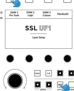
STEP 1: Enter UF1 Layer Mode by pressing & holding the 360° key.
