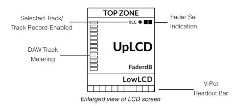
Top Zone - Provides a label for the function assigned to the soft key button directly above.
