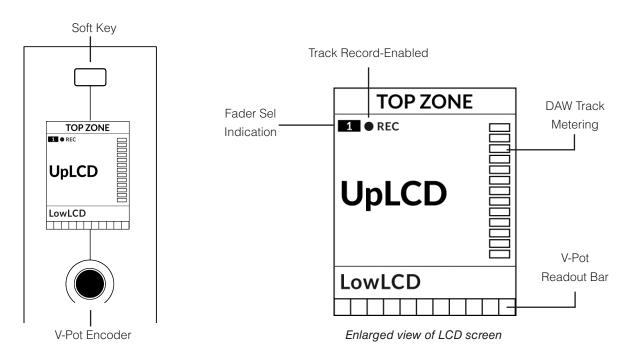
Top Zone - Provides a label for the function assigned to the Soft Key button directly above.
