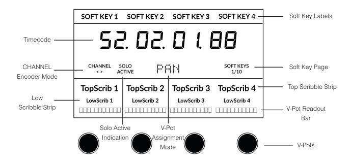
Soft Key Labels - Labels for the functions assigned to the soft keys directly above.
