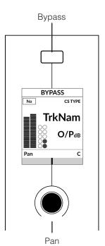
Bypass - Indicates if the channel strip is bypassed. You can toggle the bypass state from the soft key directly above.
