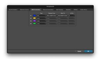
STEP 5 : Configure the UF1 unit as a HUI type. Set Receive From as SSL V-MIDI Port 1 and Send To as SSL V-MIDI Port 1.
