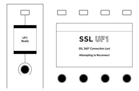
The LCD message above means that communication between SSL 360° and UF1 has been lost. If you experience this, then check that your USB cable connecting UF1 and 360° has not been removed. Re-connect if so.
