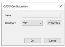
STEP 6 : Click on the Properties button. In the OASIS Configuration window, set the Transport to EMC.
