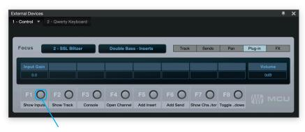
Right-click on the button and click 'Assign Command...' to change the function of any of the F keys.
