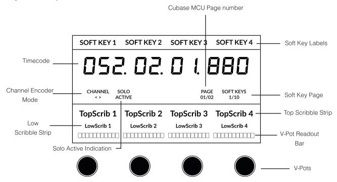
**Soft Key** - Provides a label for the function assigned to the soft key directly above.
