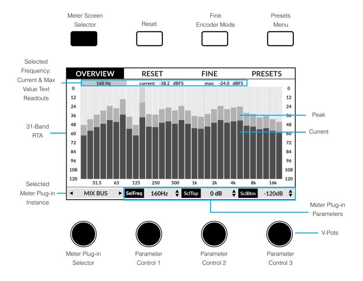
Meter Screen Selector - Press the key to toggle through the 3 different meter screens: Overview, Analogue and RTA.
