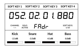
Above shows the DAW Faders "FAdr" mode has been selected. The V-Pots beneath the large screen control DAW fader levels.
