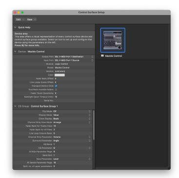
STEP 7: Set up the UF1 as a Mackie Control Unit, then assign the relevant V-MIDI Port Destination & Source for the Input & Output device.
