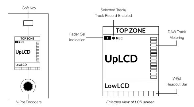
**Top Zone** - Provides a label for the function assigned to the soft key directly above.
