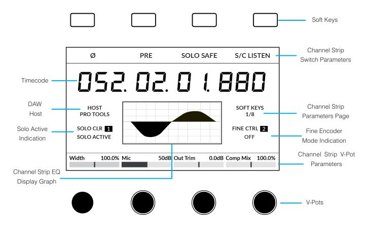
Soft Keys - Controls the channel strip switch parameters displayed directly below.
