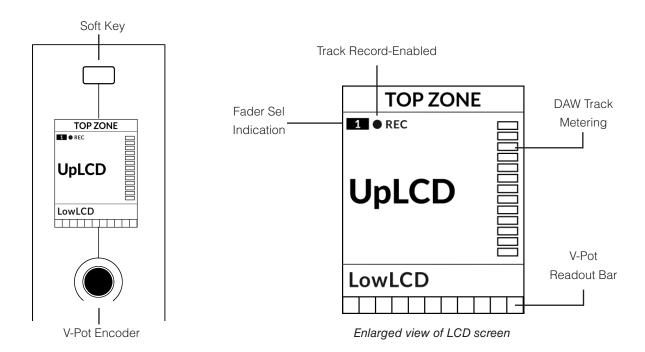
**Top Zone** - Provides a label for the function assigned to the Soft Key button directly above.
