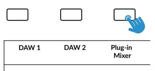
Press and hold the 360° button and whilst keeping it held down, you can switch to a different Layer by pressing the relevant top-row soft key.
