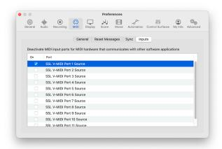
STEP 6: Enable SSL V-MIDI Port(s) in Logic. If you're working with a version of Logic that precedes 10.5, then skip this step.
