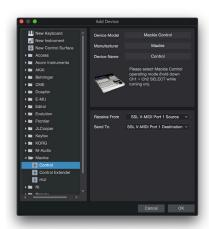
STEP 4: Add a Mackie Control and configure for SSL V-MIDI Port 1 on Receive From and Send To.
