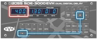
Switching Between DDL 1 and DDL 2 on the Parameter Setting Screen
