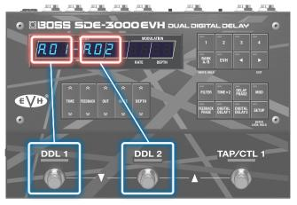
Selects and turns on/off the odd-numbered memories even-numbered memories
