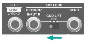
To lift the ground from the RETURN jack, move the switch to the right side (SEND).
