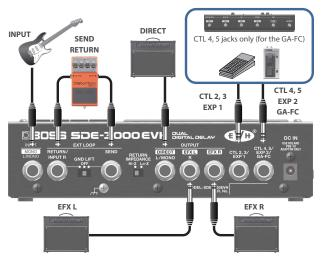
There are many other ways to connect the SDE-3000EVH. For details, refer to "Connecting an Amp and Configuring the Input/ Output Settings" (p. 12).
