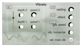
depth 1 and speed 1; when the fader reaches to two-thirds, the amplitude and speed of the vibrato will be controlled by depth 2 and speed 2.
