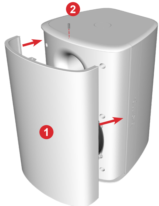
Figure 18. Reassemble the loudspeaker, carefully insert grille tabs and sides into the cabinet then re-install screws.
