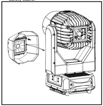
3. Loosen the screw that holds the lamp in place. Unplug the leads and lift the lamp out of its recess. Connect leads to the new lamp (same model), and place into the lamp recess.
