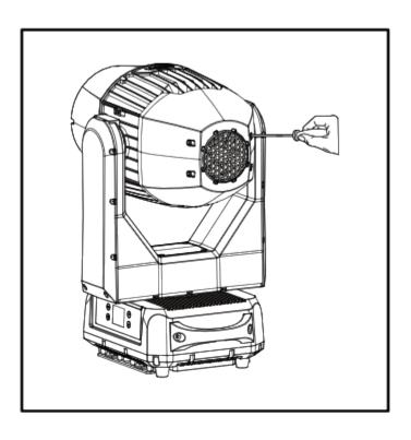
2. Loosen the screws on the head of the fixture and open the fixture head covers. Unplug the fan and loosen the screw that secures the safety cable.
