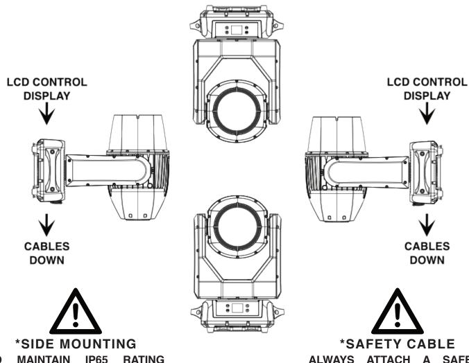
**MAINTAIN IP65** INTEGRITY, BE INSTALLED WITH FACING THE GROUND AT ALL TIMES. WATER MUST EASILY RUN OFF AND NOT COLLECT AROUND CABLE CONNECTIONS.
