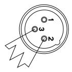
A DMX512 terminator reduces signal errors, avoiding most signal reflection interference. Connect PIN 2 (DMX-) and PIN 3 (DMX+) of the last fixture in series with a 120 Ohm, 1/4 W Resistor to terminate the DMX512.
