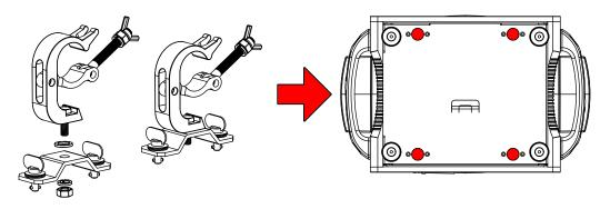
Tighten the quick-lock fasteners fully clockwise. Pull the safety-cable through the opening located on the bottom of the unit and over the trussing system or a safe fixation spot. Insert the end in the carabiner, and tighten the safety screw.
