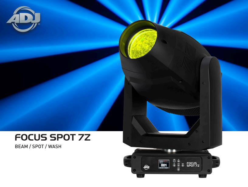
Part of ADJ's popular Focus Series of LED-powered moving head luminaires, the Focus Spot 7Z is a potent and feature-rich spot fixture. Its light source is an efficient 420W white (8,000K) LED engine, which has an average operational life of 20,000 hours. Focused through precision-engineered optics, it allows the fixture to generate a bright, punchy and even output of 20,000 Lumens.
