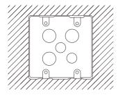
2. Connect CAT5-STP cable, then install the panel into the 2 gang box and tighten it with accessory screws.
