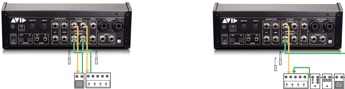
Connecting two mono guitar pedals to FX Loops 1–2 (shown at left) and multiple pedals in series to a single FX Loop (shown at right)
