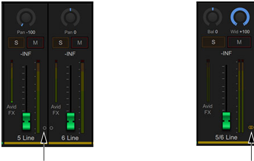
Channel Link button in unlinked channels (Line In 5 and 6, shown at left) and linked (shown at right)
