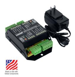
General purpose relay module with two (2) double pole double throw (DPDT) relays serves as a reliable building block in a wide variety of applications.
