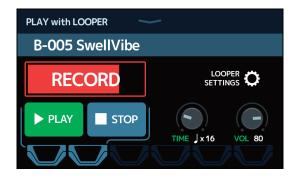
Looper settings can be made and recording and playback can be started and stopped using the touchscreen and footswitches.
