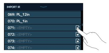
Impulse response data is already assigned to locations 001–106. You can assign impulse response data as you like to 107–300.
