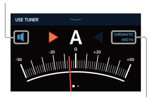
This shows the tuner type and standard pitch. Touch this to change tuner settings.
