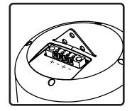
**2.** Connect signal wire to screw-down terminal block. Tighten unused terminal screws. Use inside positive and negative inputs for either voice coil or distributed systems.
