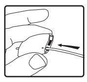
**4.** Thread hanging or safety cable through SpeedClamp™ mechanisms as shown.
