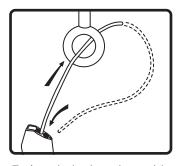
**5.** Attach the hanging cable by securing it and the safety cable to structure as shown.
