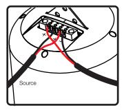
**3.** When daisy chaining, wire the outside terminals to the inside terminals of the next speaker. This step only applies to tap settings using the transformer and not when the speaker is used on bypass.
