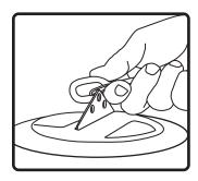
**9.** Attach the safety cable to one of the secondary holes in the hanging bracket.
