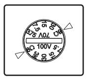
**1.** Remove the magnetically-attached grille from the front of the speaker to reveal the rotary tap switch. Select tap position on rotary switch. Switch is preset to maximum tap setting in 70.7V mode.
