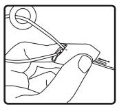
**6.** Thread cable end(s) through SpeedClamp™ mechanisms as shown.
