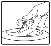
**8.** Attach hanging cable to the center hole in the speaker hanging bracket.
