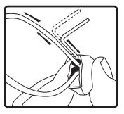
**7.** Adjust speaker hanging height with SpeedClamp™ mechanism. Pull to tighten & insert release key (small hex wrench) into SpeedClamp ™ as shown to loosen or adjust.
