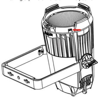
3. While holding the latch in place, slide the desired lens into place. Then release the latch. It will automatically move back into the locked position when released.
