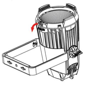
2. Push the latch towards the location of the retaining clip. Hold the latch in this position.
